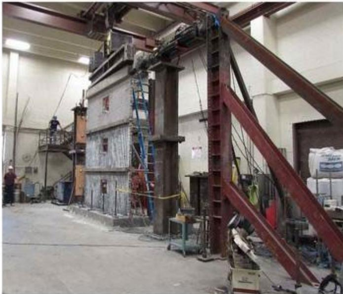
Figure 4 - : Reaction/Testing Frame
