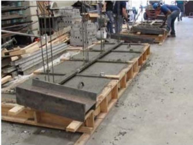
Figure 1 - Reinforced concrete footing
