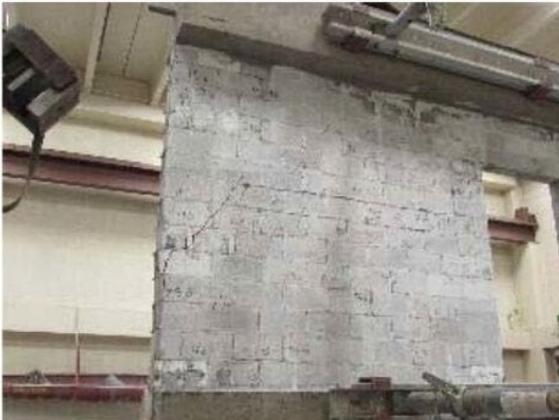
Figure 8 – Failure of Wall 5
