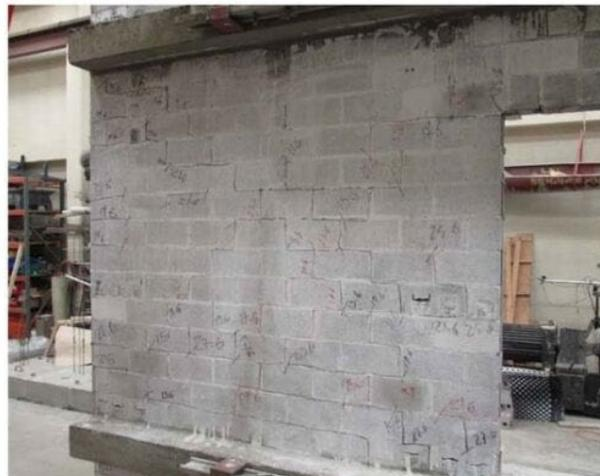
Figure 6 – Crack Pattern
