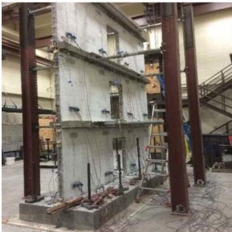
Figure 5 - Instrumentation
